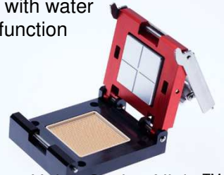
Union Socket Ninja™ Semi-custom-made test socket
